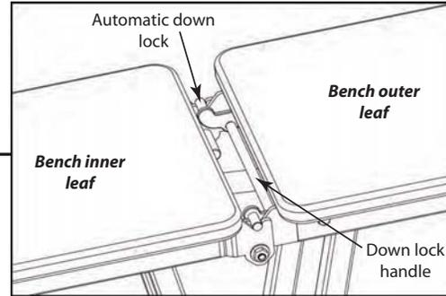
**Down lock** automatically engages when table and bench are lowered to floor to prevent accidental tip up. **Bench design does not 'jackknife' if tipped onto its side.** Manual disengage by lifting up on lock bar and outer leaf when returning to **storage cabinet**.
