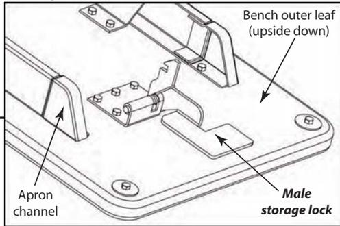
Leaf to leaf **storage lock** automatically engages when table or bench is pushed into **storage cabinet**. Manual unlock with hand or **release handle**. The release is located at the bottom of the outer leaf when in the **storage cabinet**.
