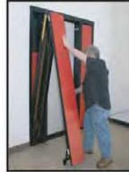
3) Keep both hands on bench while pulling out with lower hand and stabilizing bench with upper hand. **Do not pull down from top of bench!**
