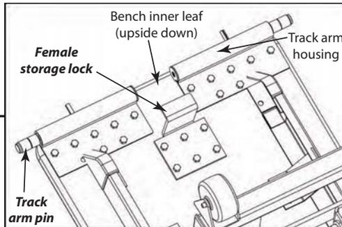
Secure the table and bench inner leaves to cabinet **post tracks** for storage. Spring loaded manual pin extends for storage and retracts for removal from **storage cabinet**.
