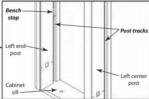
Post tracks capture **track arm pins** securing inner table and bench leaves to **storage cabinet**. **Bench stops** prevent accidental bench tipping when benches are attached to **storage cabinet**.
