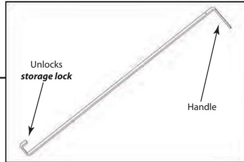
Releases **storage lock** centered at the bottom of tables and benches when in **storage cabinet**. **To unlock:** Insert under unit at the center of leaf and tilt handle away from cabinet.
