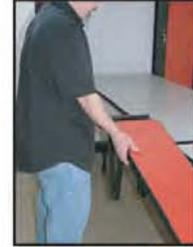
4) When unit is stable in the 'tee-pee' position face side of bench placing a hand on each leaf top. **Check that automatic down lock is engaged!**
